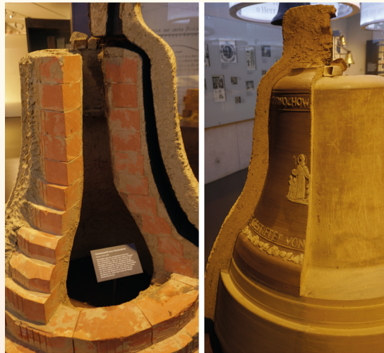
Model of a bell casting mold, combining many steps from the production of a mold for the manufacture of bronze bells
